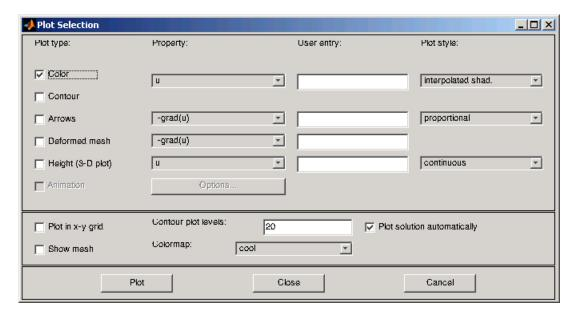
For eigenvalue problems, the bottom right part of the dialog box contains a pop-up menu with all eigenvalues. The plotted solution is the eigenvector associated with the selected eigenvalue. By default, the smallest eigenvalue is selected.
