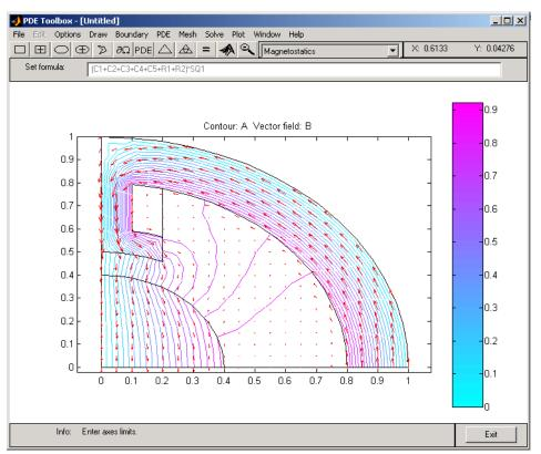
Equipotential Lines and Magnetic Flux in Two-Pole Motor
