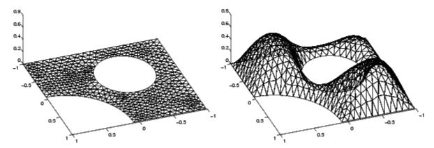
A Triangular Mesh (left) and a Continuous Piecewise Linear Function on That Mesh
