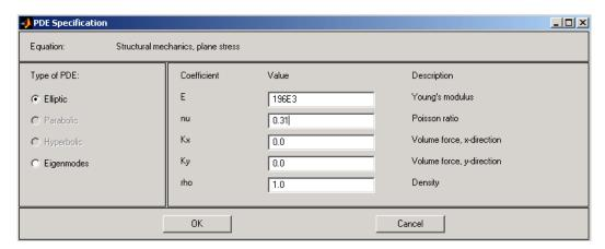
The E and [[v (nu) parameters are Young's modulus and Poisson's s ratio, respectively. There are no volume forces, so Kx and Ky are zero.  $\rho$  (rho) is not used in this mode. The material is homogeneous, so the same E and [[v apply to the whole 2-D domain.
