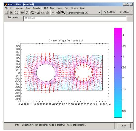
The Current Density Between Two Metallic Conductors
