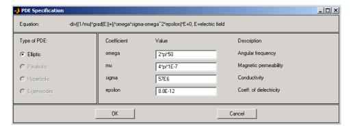
Initialize the mesh and solve the equation. Due to the skin effect, the current density at the surface of the conductor is much higher than in the conductor's
