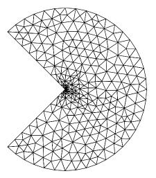
The maximum absolute error is 0.0058, with 534 triangles. We test how many refinements we have to use with a uniform triangle net:
