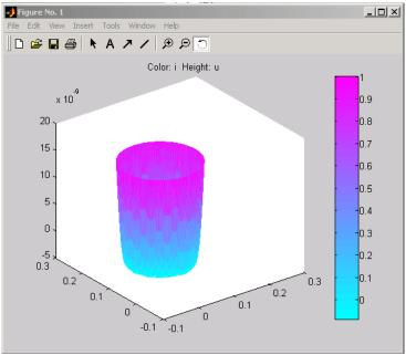
The Current Density in an AC Wire
